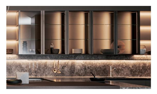
Flair wall units are made with a 19 mm thick aluminium frame, in titan or pewter finish. The doors are available in three tempered 4 mm thick glasses: transparent extra-clear, fumé and bronze. The internal shelves are available in melamine, lacquer, wood or glass finish. The doors can be opened thanks to a small handle in the lower part of the door.
